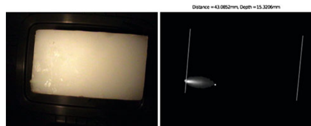
Fig. 1 (a) Illuminated frame from tissue penetration phantom. Chemoluminescent agent is illuminated however not visible. (b) Illustration of the segmented chemoluminescent agent within the tissue phantom. The vertical lines represent the edges of the phantom segmented through manual methods. The white dot is the point at which the penetration depth was measured
