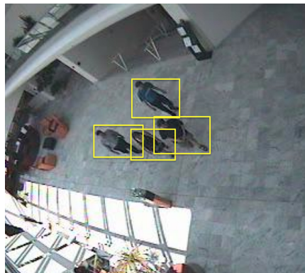
Figure 6. Detected individuals in a frame from EU CAVIAR video sequence.
