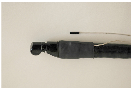
Figure 1. Position sensor placed next to endoscope tip to show relative size. The sensor is glued to the endoscope tip and covered with shrink-wrap tubing.
